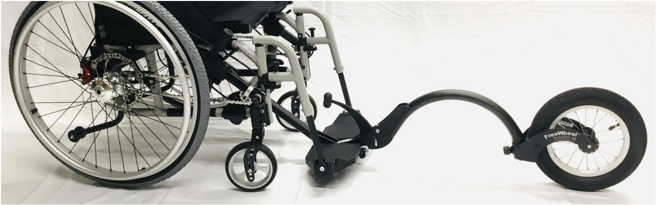
FreeWheel Attached to Jackdrive TNC+ with The FreeWheel in Forward Facing Mounting Position
